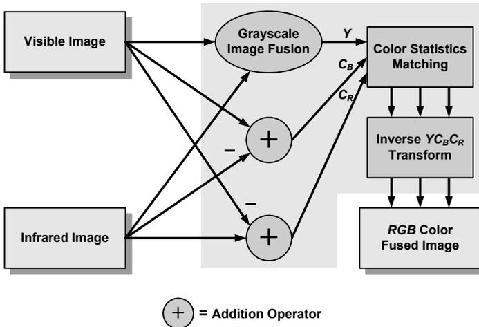
Fig. 1. Fusion architecture of the AOCT method
