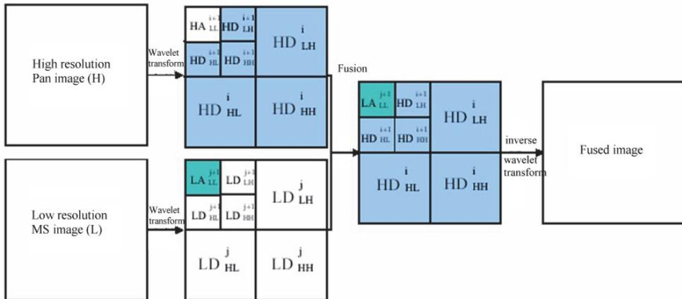
Fig. 4. Generic flowchart of wavelet-based image fusion
