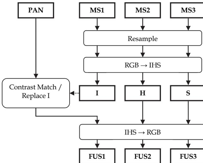
Fig. 1. Block scheme of the IHS fusion method.
