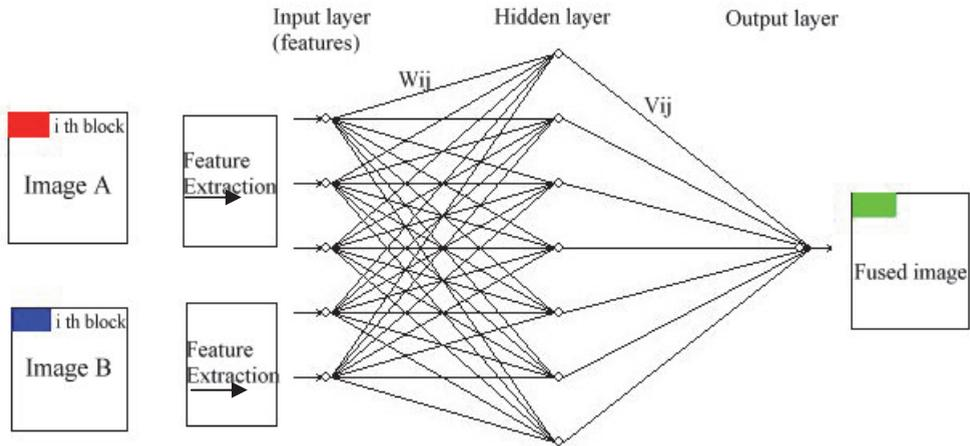
Fig. 6. General schematic diagram of the ANN-based image fusion method.
