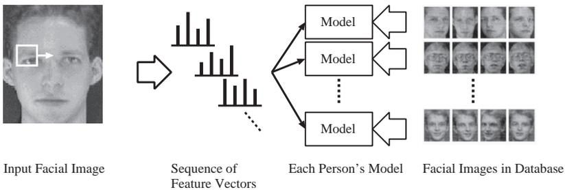
Fig. 18. Pseudo-2D HMM-based face identification system. A sequence of feature vectors is generated from the partial image in the scanning window, which is then matched with each person's HMM using the Viterbi algorithm. Then, the maximum-likelihood model yields the identity of the face.
