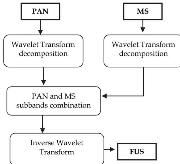
Fig. 3. Block scheme of the WT fusion method.
