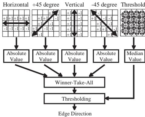
Fig. 2. Procedure of directional edge extraction.
