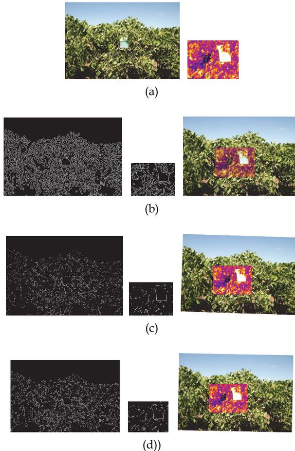
Fig. 7. Tests of variable resolution algorithm based on different edge extraction methods (a) Optical raw image(left) and infrared raw image(right), (b) Results of edge extraction using Canny algorithm(left) and registration result (266,254,-0.4), (c) Results of edge extraction using Roberts operators(left) and registration result (265,253,1.8), (d) Results of edge extraction using Sobel Operators(left) and registration result (265,256,1.1)
