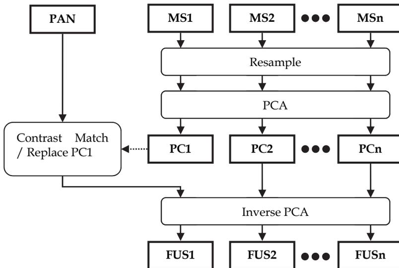
Fig. 2. Block scheme of the PCA fusion method.
